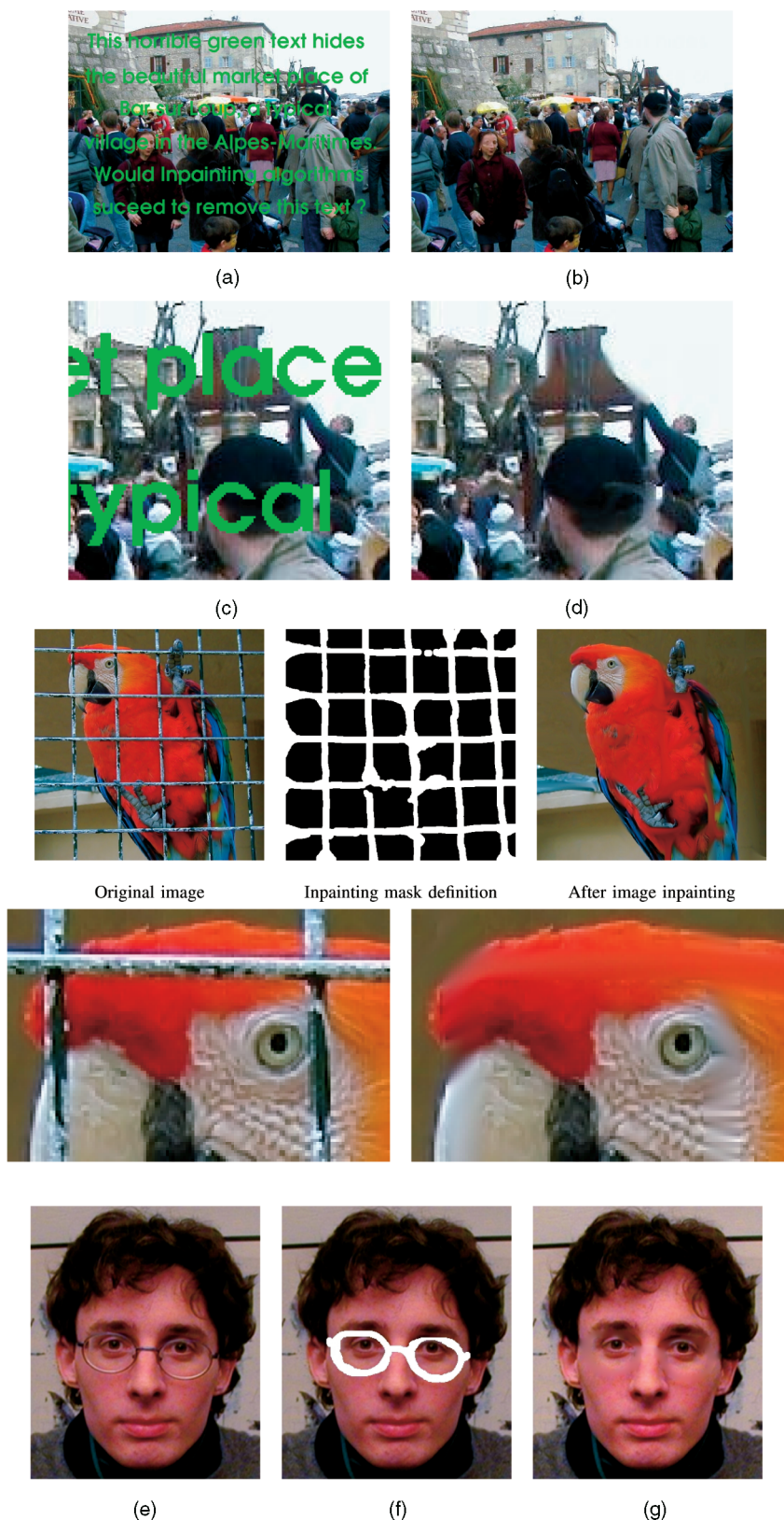
Fig. 10. Using vector-valued regularization PDE's for color image inpainting (2). (a) Image with undesired text. (b) Inpainted color image. (c) Zoom of (a). (d) Zoom of (b). (e) Original color image. (f) Image + Inpainting mask. (g) Inpainted image.
