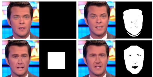
Figure 1. Original video frame (top left), video frame modified using Face2Face method [30] (top right, smooth mask almost completely covers the skin area), using Deepfakes method [1] (bottom left, rectangular mask), and using FaceSwap method [27] (bottom right, polygon-like mask).
