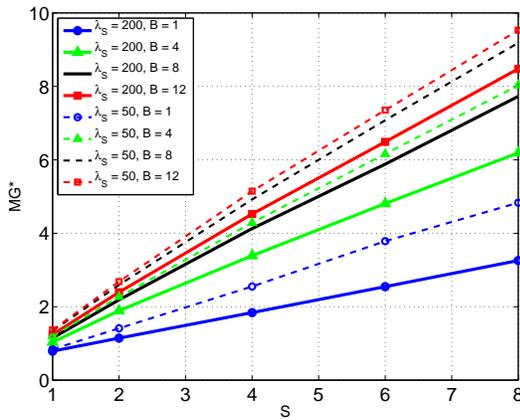
Fig. 5. Scheduling user intensity optimized area multiplexing gains per pilot dimension as a function of the UL pilot beam-width and the number of RRH sectors (geometric RRH sectorization).
