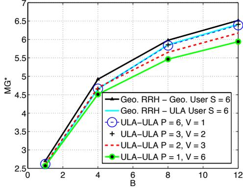
Fig. 7. Scheduling user intensity optimized area multiplexing gains per pilot dimension as a function of (nominal) UL pilot beam-width ( $360/B$  degrees) for the practical sectorization designs in Fig. 6.
