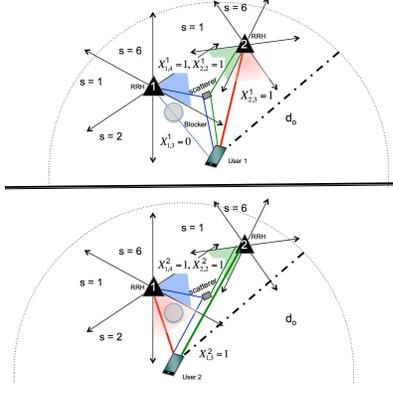
Fig. 1. Two RRHs are shown within  $d_o$  distance from the two UTs. The first and the second RRHs are, respectively, represented by the triangles 1 and 2. Each RRH employs 6 sectors. Also shown are a single scatterer and a single blocker.
