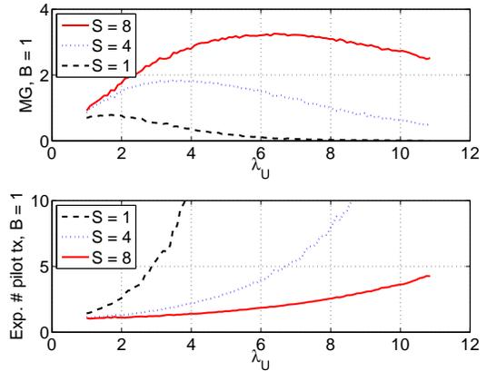
Fig. 3. Top figure: Area multiplexing gains per pilot dimension vs. scheduling user intensity (omni UL pilots). Bottom figure: Expected number of UL pilot transmissions per delivered packet vs. scheduling user intensity (omni UL pilots).
