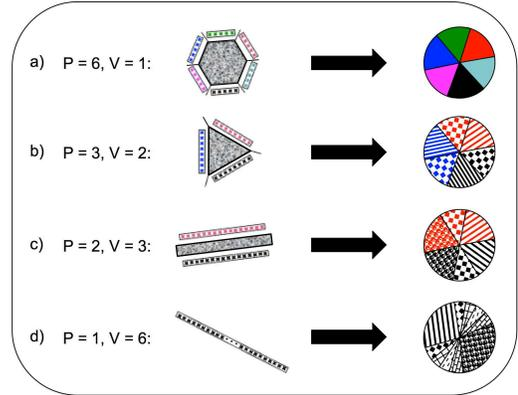
Fig. 6. Practical sectorization designs (left) and associated sectorization patterns (right).
