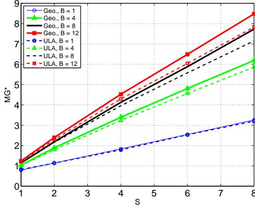
Fig. 8. Scheduling user intensity optimized area multiplexing gains per pilot dimension as a function of number of RRH sectors and UL pilot training beam width: geometric (solid) and ULA based (dashed) sectorization.
