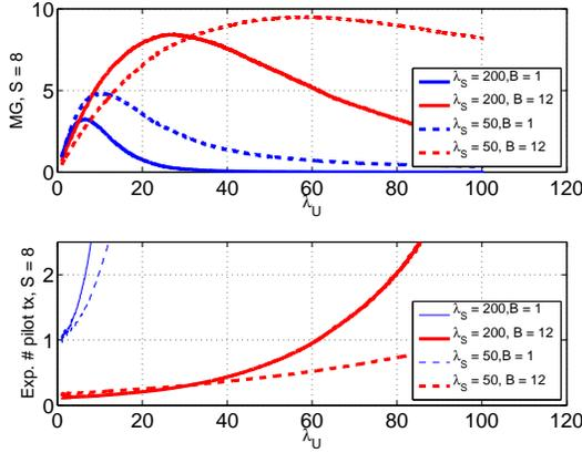
Fig. 4. Top figure: Area multiplexing gains per pilot dimension vs. scheduling user intensity. Bottom figure: Expected required UL transmit power per delivered packet vs. scheduling user intensity. In both figures  $S = 8$ .
