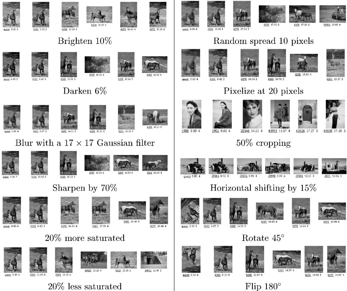
Fig. 16. The robustness of the system to image alterations. Due to space, only the best five matches are shown. The first image in each example is the query image. Database size: 200,000 images.
