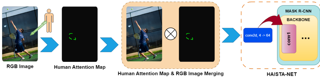
Figure 2: Method Outline. Users draw a couple of pixels according to their attention to the object. Then, a Human Attention Map is generated to concatenate with the RGB image to feed the model. We denote the concatenate operator as \otimes .
