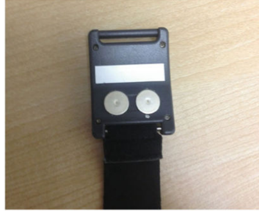
b Back of sensor, showing skin electrodes
