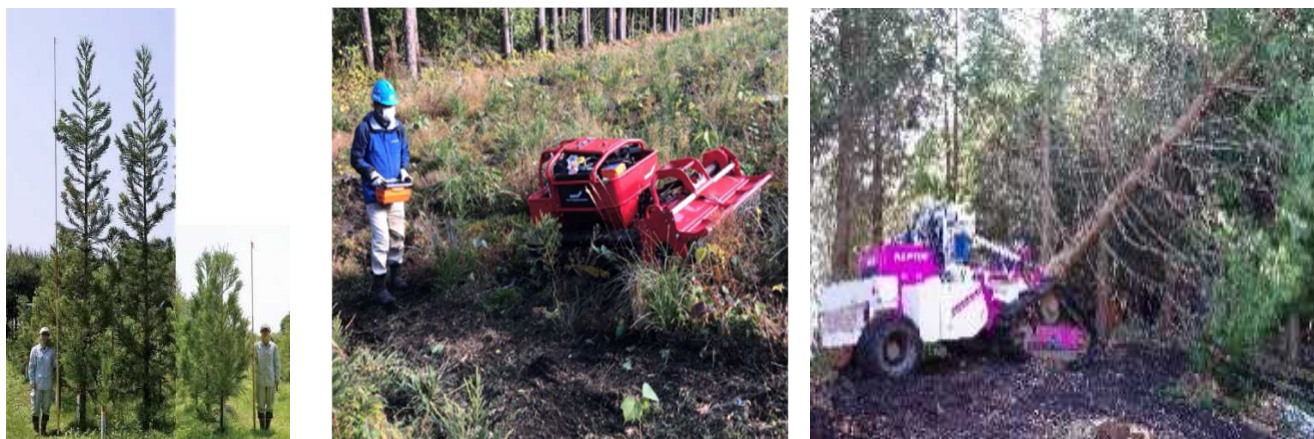
Figure 30 Examples of low-cost and labor-saving forestry operations through forestry innovation (Left: Introduction of “elite tree” species, etc.; Middle: Remote-controlled multi-purpose forestry machines for clearing and transporting seedlings; Right: Remote-controlled logging and conveyance) (Source: Ministry of Agriculture, Forestry and Fisheries)
