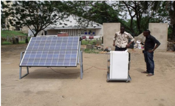
Experimenting with a solar PV-powered vapour-compression refrigerator in Nigeria. Photo credit: [86]
