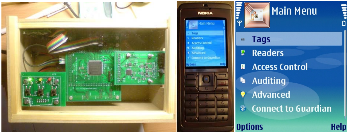
Figure 15: Privacy Guardian Reader Hardware and User Interface © 2006 M. Rieback. Images reprinted with permission from http://www.rfidguardian.org
