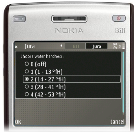
Fig. 2. Detailed view of an applet that lets users control their coffee maker. The screenshot shows how the coffee maker’s water hardness settings can be adjusted.
