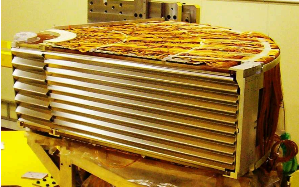
Figure 3.10: photograph of an EMEC module, showing the accordion structure of the absorbers. The boundary between the inner wheel and the outer wheel can be seen towards the left, where the shape of the absorber plate changes.
