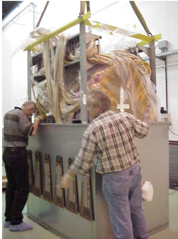
Figure 4.4: Photograph of the FCal being lowered into the bathtub used for the beam test. The polyethylene used to simulate the plug portion of the ATLAS JM shielding is visible on the front of the bathtub, while the summing boards can be seen on the left side.
