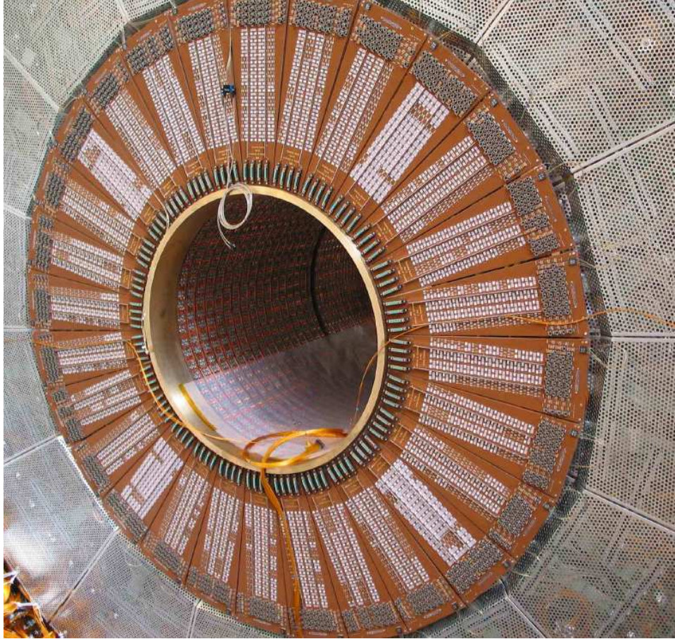
Figure 3.15: The FCal summing boards mounted on the rear of the HEC[45]
