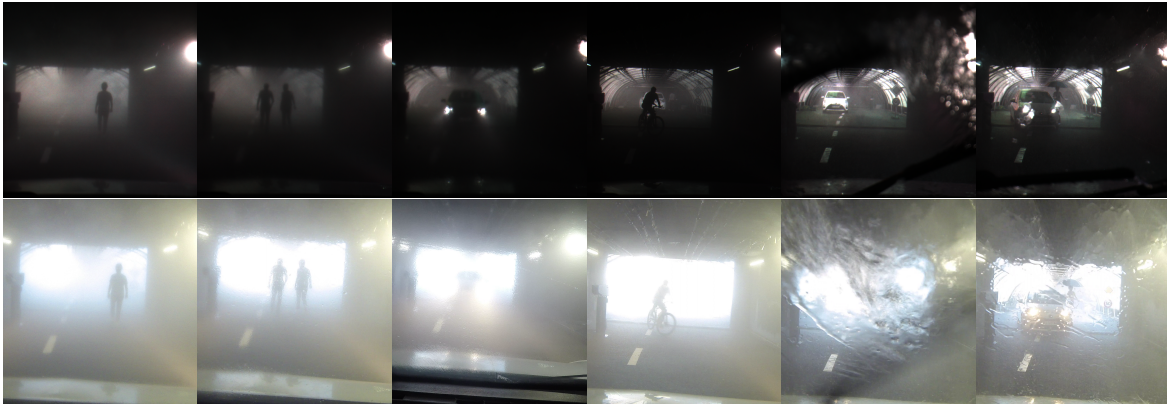
Figure 4.5: Examples of road scenes captured during the multimodal acquisition campaign at the Cerema tunnel. First row contains the the polarimetric version of the scenes, represented by the intensity images I = (I_0, I_{45}, I_{90}) , and second row is their RGB equivalent.
