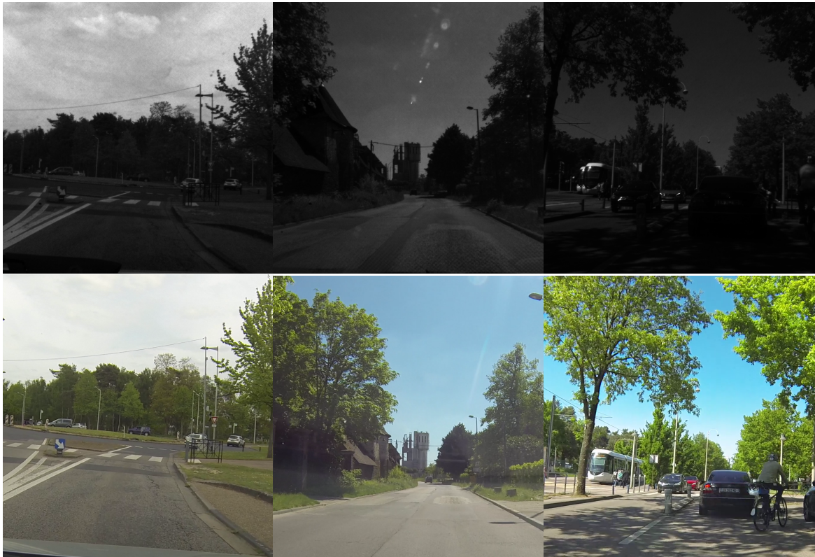
Figure 6.4: Illustration of the offset variation. The first row is the polarimetric images represented by I_0 and the second row their RGB equivalent. In the first column, the polarimetric and RGB images are almost stackable whereas in the second and third columns a slight temporal offset is noticed between the RGB and polarimetric images.
