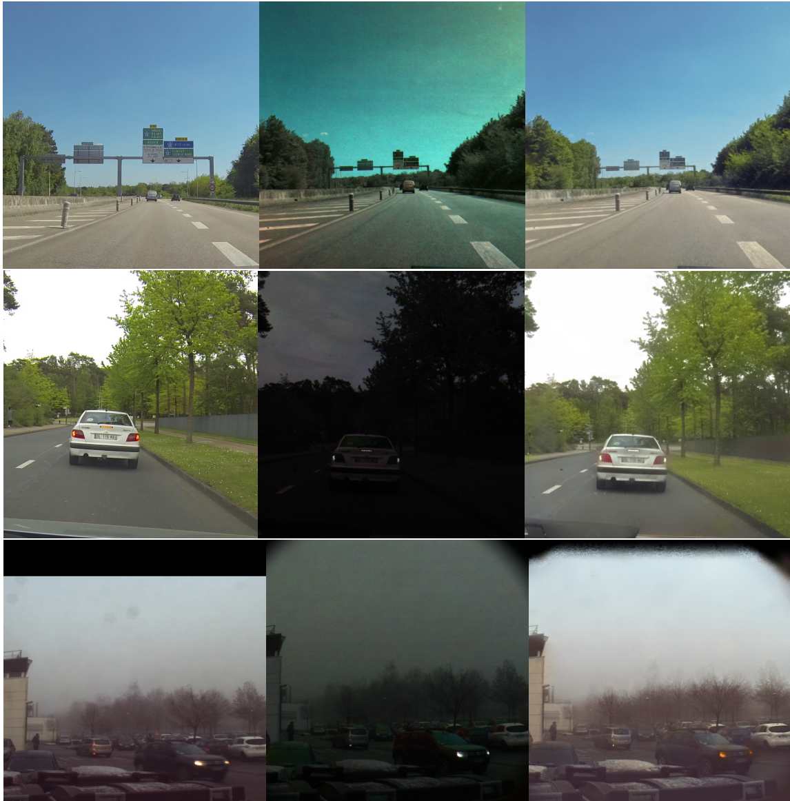
Figure 6.6: Example of registered images using a CycleGAN. The first column contains the real RGB images, the second column contains polarimetric intensities images I and the third column contains the RGB images that are registered towards I .
