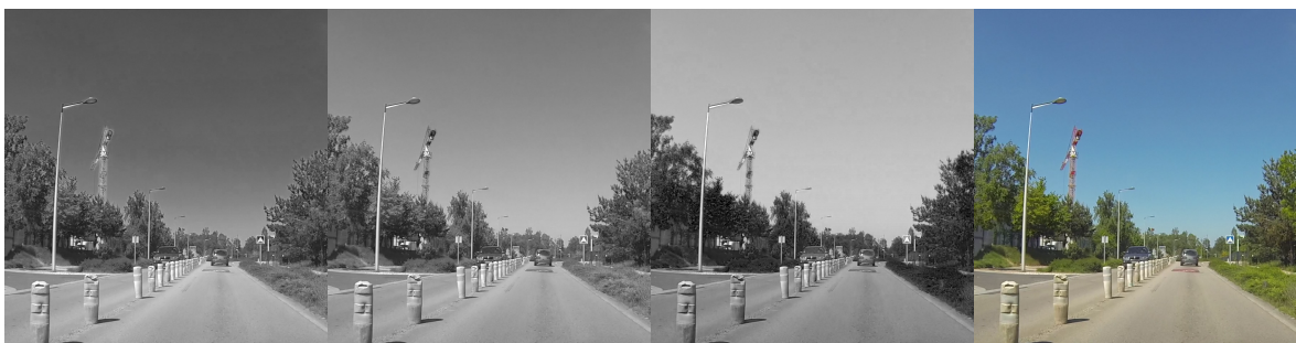
Figure 1.8: Example of an RGB image and its channels decomposition. From left to right, the red channel, the green channel, the blue channel and their concatenation to constitute an RGB image.
