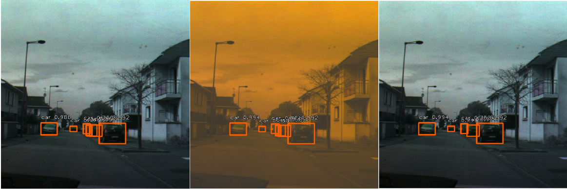
Figure 6.2: From left to right, the detections on the intensities images I = (I_0, I_{45}, I_{90}) , on the Pauli inspired images \text{Pauli} = (S_1, I_{45}, S_0) and the fusion of these two modalities using a naive NMS filter. A loss of information can be noticed regarding the prediction of the fused modalities when cars are parked one behind another. This is due to the suppression of close bounding boxes when the naive NMS filter has to process too many of them.
