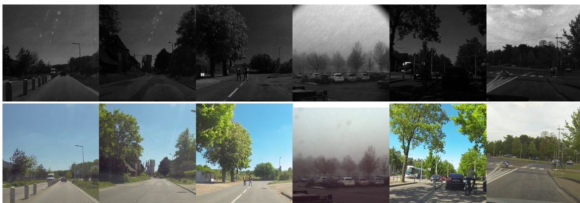
Figure 4.4: Examples of road scenes captured during the multimodal acquisition campaign. First row contains the the polarimetric version of the scenes, represented by the intensity I_0 , and second row is their RGB equivalent.
