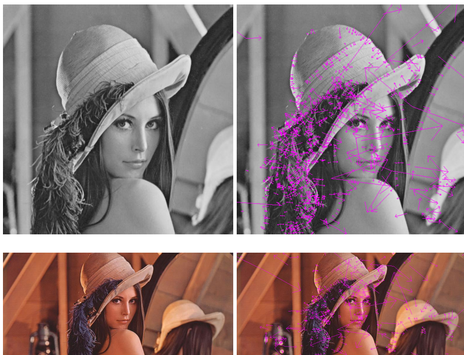
Figure 2.1 – SIFT – Keypoints Detection. Top image: 1128 detected keypoints on a 512 \times 512 pixels image. Bottom image: 519 detected keypoints on a 780 \times 350 pixels image (Generated using OpenSIFT Library).
