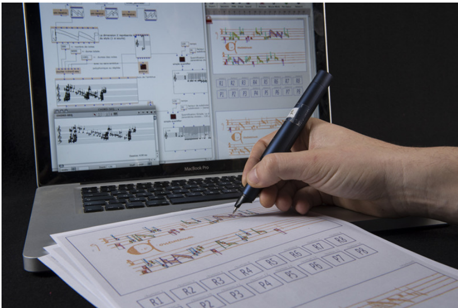
Figure 7.4: Exploring computer-based musical processes on paper. Pen events on the paper interface trigger musical processes in OpenMusic which generate direct audio-visual feedback. Photo H. Raguet ©Inria.
