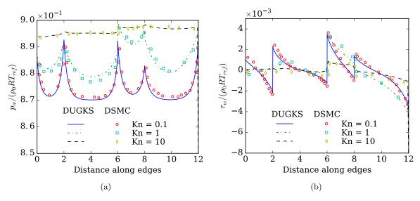
Figure 7: Non-dimensional normal stress (a) and shear stress (b) along the surface of the microbeam. The x-axis represents the path length along the microbeam surface starting from the left-upper corner with a counter-clock direction.
