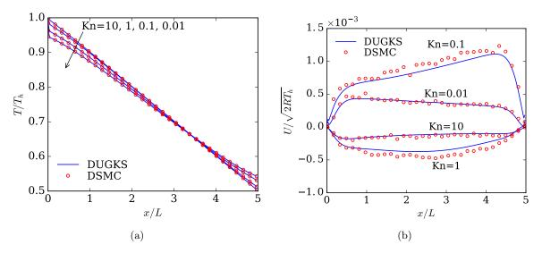
Figure 4: Non-dimensional temperature (a) and U-velocity (b) profiles along the horizontal center line of the therm creep flow case.
