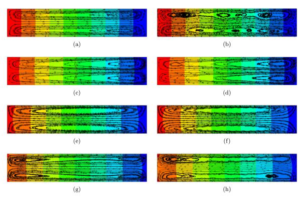
Figure 2: Temperature contours and streamlines for the thermal creep flow case. Left panel: DUGKS results. Right panel: DSMC results. Knudsen numbers in each panel from top to bottom are Kn = 0.01, 0.1, 1 and 10. The non-dimensional contour levels in each contour plot are from 0.65 to 0.95 with a uniform step of 0.05.
