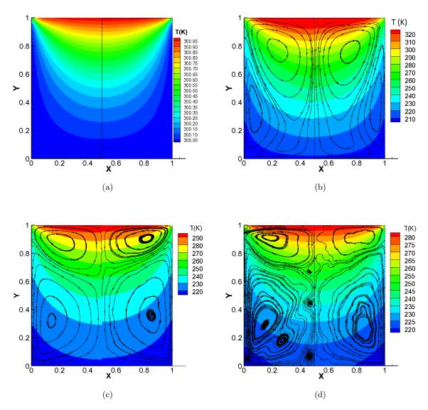
Figure 12: Temperature field and streamlines [only in (b), (c), (d)] of the temperature discontinuity induced flow case. Sub-figure (a) is for the case of Kn = 0.001, left and right half are the DUGKS solution and the analytical solution based on heat equation [(24)]. Sub-figures (b), (c) and (d) correspond to the cases of Kn = 0.1, 1 and 10, respectively. In each sub-figure, left and right half are results using the DUGKS and DSMC method, respectively.
