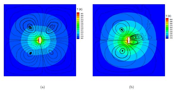
Figure 9: Temperature field and streamlines of the radiometric flow case. Left: Kn = 1. Right: Kn = 0.1.
