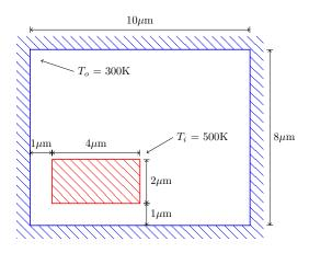
Figure 5: Heated microbeam (cross section) in a cavity.
