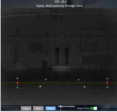
Fig. 4. Scene calibration: Calibration markers in green are labelled (sagittal view). Walking line is defined between the start and end points, shown in red.
