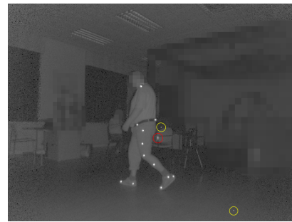
Fig. 2. Noise from the sensor (yellow) and reflective material (red)
