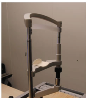
Figure 24. Chinrest. A chinrest is required in all tests to ensure the eye positions remain constant throughout the test series.
