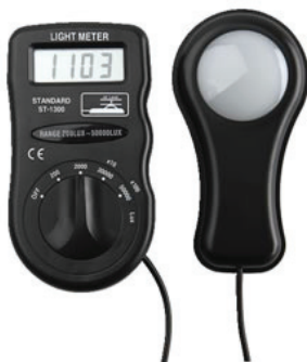
Figure 23. light meter. A light meter is required in order to determine the illumination in the test lab.
