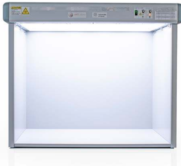
△ Figure 1: New LED light box at SSEF that was developed in collaboration with the Electronics Department, University of Basel. The new light box adheres to the requirements set out in the new standard ISO 24016 and is more comfortable to work with than conventional light sources for colour grading. Photo: L. Phan, SSEF.
