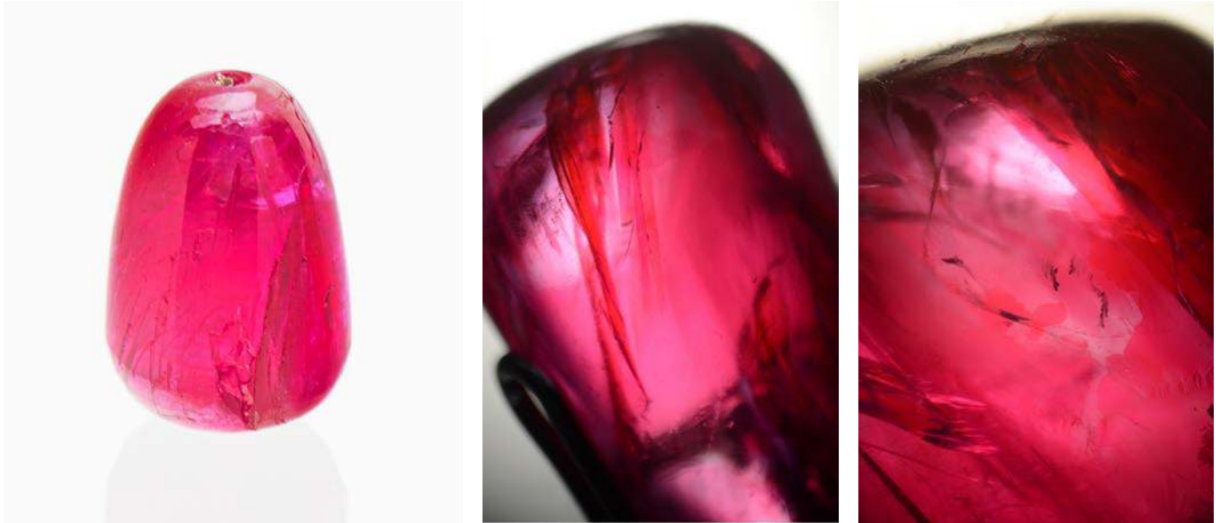
△ Figure 1 (left): Dyed corundum from Burma (Myanmar), mimicking a beautiful pinkish red ruby. Photo: J. Xaysongkham, SSEF. Figure 2 (center and right): Fissures filled with red oil in this treated (dyed) corundum. Photos: M.S. Krzemnicki, SSEF.
