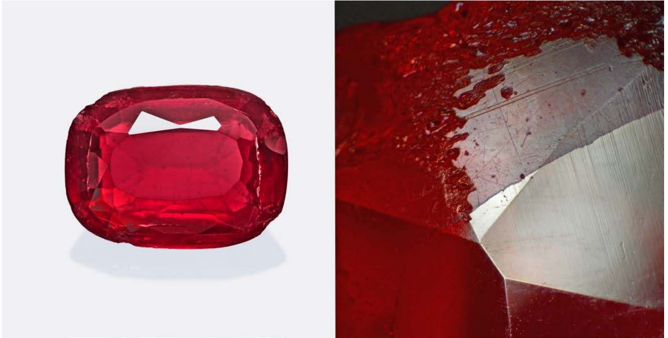
△ Figure 1: This red garnet-topped doublet is already obvious when looking carefully on the stone. Even more so, when checking the lustre difference of the garnet top and the glass base under the microscope (magnification 35x). Photos: M. Bichsel & M.S. Krzemnicki, SSEF.
