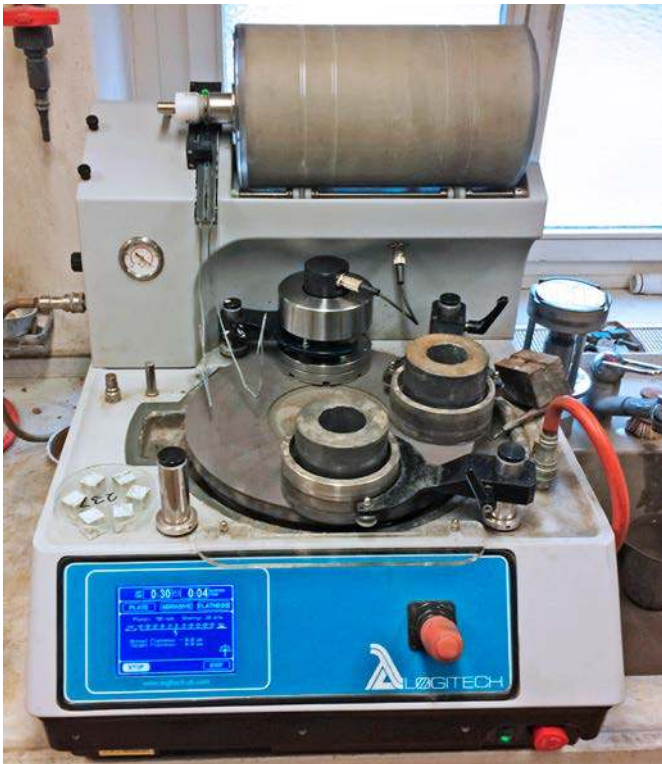
△ The lapping machine from Basel University charged with sample cubes for the relative grinding hardness measurements. Photo: H.A. Hänni.
