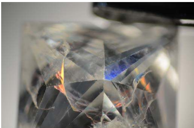
△ Figure 2: Beautiful flash effect seen under microscope in this fissure-filled diamond, but not nice as it was not disclosed! Photo: SSEF.
