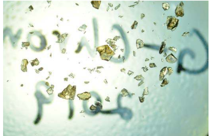
△ Figure 1. Tiny fragments of the 'Rak-17' zircon. The largest fragment is about 1.5mm in size. The GemTOF analyses at SSEF were carried out on a random selection of these fragments. Photo: SSEF.
