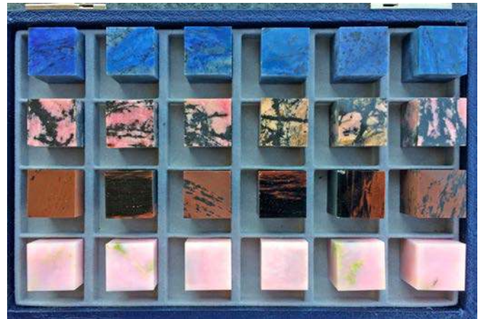
△ Sample cubes of ornamental stones for grinding hardness (GH) measurements in preparation. Photo: H.A. Hänni.
