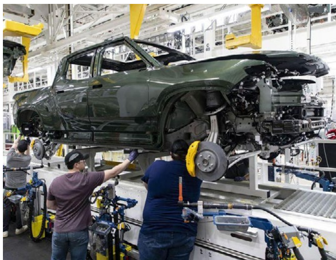
Workers lower an R1T truck body onto a chassis in the assembly line at the Rivian electric vehicle plant in Normal, Ill., on 11 April 2022.
