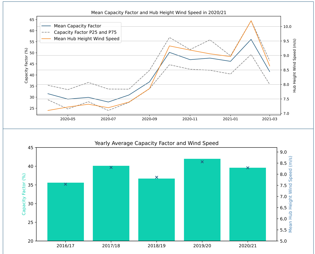
Figure 1 - Capacity factor over time in 2020/21, featuring quartile ranges and mean wind speed, (top) and capacity factor describe by financial year from 2016/17 (bottom).
