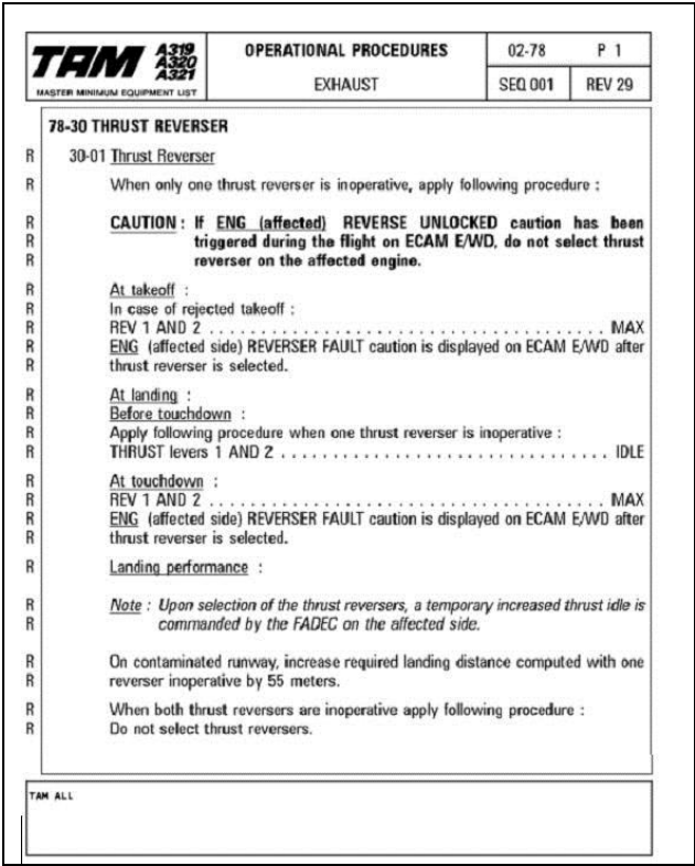
Figura 12 - MMEL A-319/320, "Operational Procedures", Rev 29, 78-30 "Thrust Reverser"
