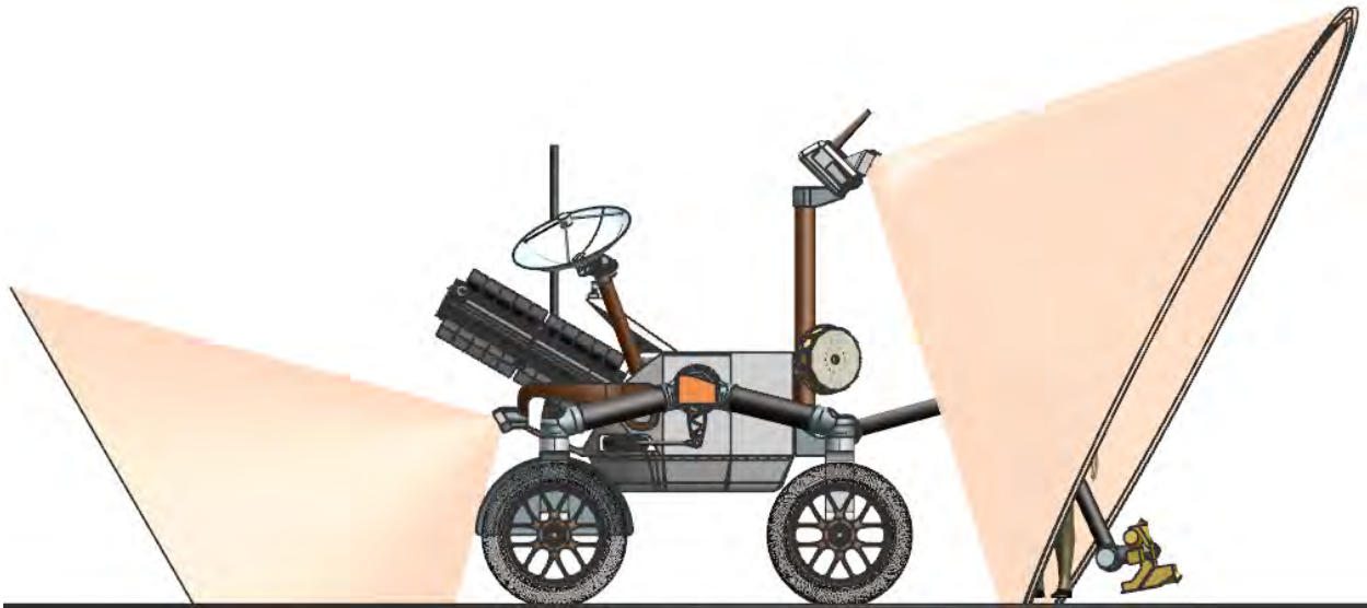
Figure L-37. Right side view of the rover with the navigation camera FOVs shown (front and rear).
