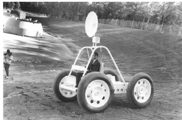
Figure D-5. An example of a lunar rover prototype with different sized front and rear wheels: the Local Scientific Survey Module (LSSM) developed in 1965 by Brown Engineering (NASA).
