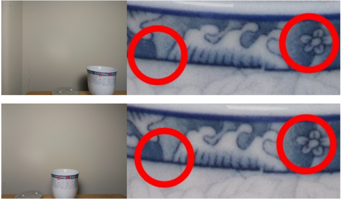
Figure 20: Left Single Camera Pair(SCP) Coordinates for: Top(Left Image) [left point (2585, 1942) : right point (2811, 1924)], Bottom(Right Image) [left point (1504, 1942) : right point (1716, 1922)]. Here (Left Image) and (Right Image) refer to the SCP in terms of a stereo pair so the formulas from equation set (13) follow. The SCP for the Top and Bottom images have a base length of 89.98mm
