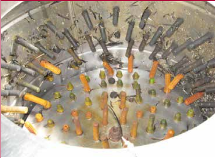
Mechanical fingers should be renewed regularly, as cracked and worn fingers can harbour bacteria
