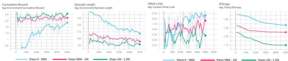
Figure 29. Level 3 – Cumulative Reward, Episode Length, Value Loss and Entropy graphical presentation for avoiding the obstacles with combined movement. There are 3 phases: steps 0 - 500,000 (blue line), steps 500,000 - 1,000,000 (red line), and steps 1,000,000 – 1,500,000 (green line). Blue, red and green lines are in a sequence of 500,000 steps each phase.
