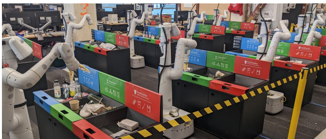
Fig. 5: The robot classroom, a controlled setting for repeatable evaluations. 20 robots continuously collect data at 20 waste stations.
