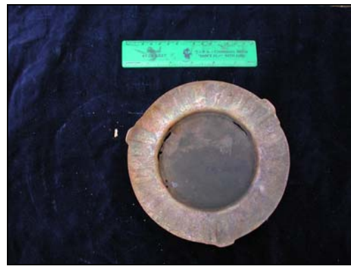
Figure C-6. 61: Underside view of 80 pr RML (possibly Palliser) automatic gun gas check plate. Scale = 20cm (Peter Ferrier Collection).
