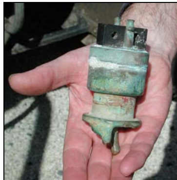
Figure C-6. 56: Electrical contact mine detonation mechanism (Peter Ferrier Collection).
