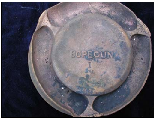
Figure C-6. 60: 80 pr RML (possibly Palliser) automatic gun gas check plate (Peter Ferrier Collection).
