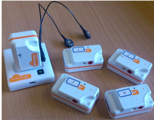
Figure 3.4. The sensor testbed composed of five identical Shimmer sensors
