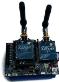
Figure 6. IoT Node deployed in SmartSantander
