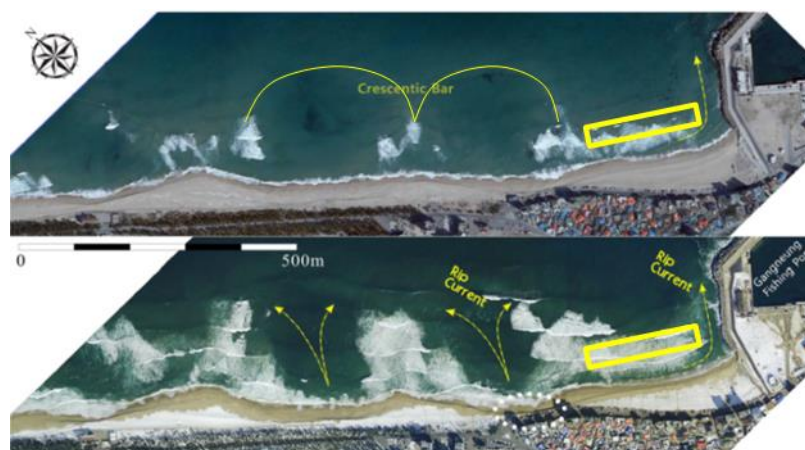
Figure 2. Presence of crescentic bars at Anmok beach with an indication of the locations where rip currents occur. The yellow rectangle represents the submerged breakwater that was constructed in 2014 at Anmok beach.
