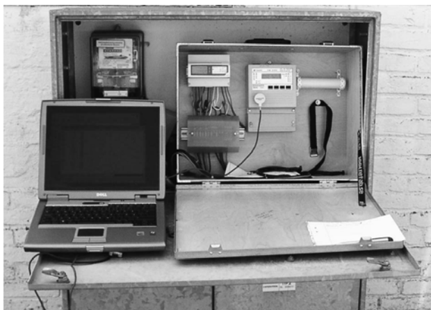
Figure 3. (Left) Measuring equipment for recording of data and (right) formula used to calculate average current consumption during a 5-minute interval. The computer was only used to collect data from the recording equipment.
