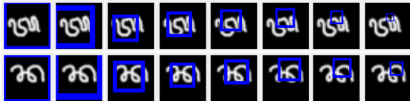
(a) It can be seen that the two characters look very similar in their stroke pattern and differ only in their looping structure. ARC has learnt to focus on these crucial aspects.
