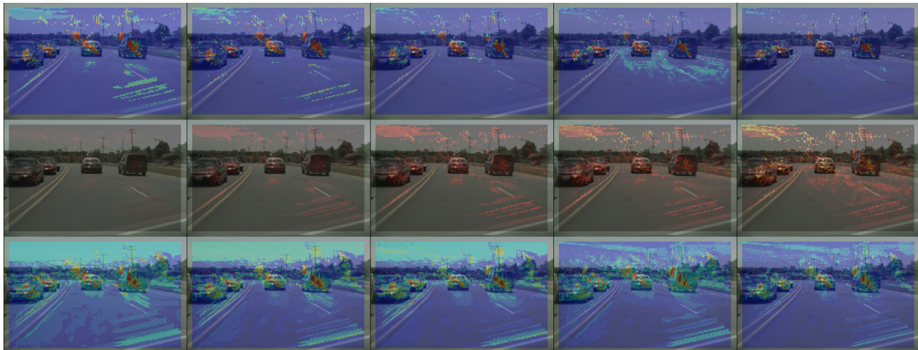
Figure 5: Images displaying the detection activations on a test image for the anytime predictor produced by SPEEDBOOST (top) and the cascade (bottom). Displayed in the middle is a heat map of the number of features evaluated by the SPEEDBOOST predictor for each pixel. Images are arranged left to right through time, at intervals of 7 average feature evaluations per pixel.
