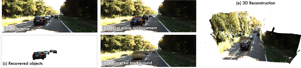
Figure 6: Scene reconstruction using our pipeline on KITTI. Our pipeline decomposes the scene into objects (c) and background (d) and recovers full geometries and appearances (e). This allows for scene manipulation, view synthesis and novel scene arrangements (b). Despite being trained on synthetic data, our pipeline generalizes well to real images without any adaptation.
