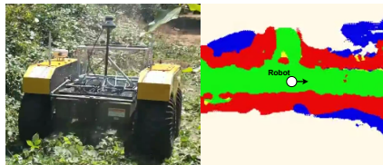
Figure 1: Example target scenario. BEVNet can be run on the Clearpath Warthog to generate semantic map of offroad environments.
