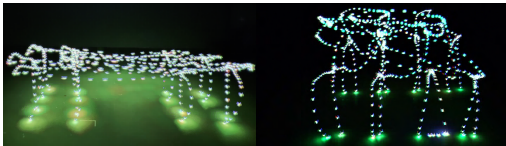
Figure 6: Time lapse of eight drones swapping goals (left) and performing a formation change (right).
