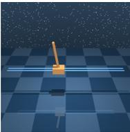
Figure 12. **Cartpole (4, 1, 5)**: **Cartpole** domain aims to control the pole attached by an un-actuated joint to a cart. In both the `swingup` task and the `swingup-sparse` task, the pole starts pointing down and aim to make the unactuated pole keeping upright upward by applying forces to the cart, while in `balance` and `balance-sparse` the pole starts near the upright.
