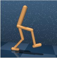
Figure 10. **Walker (18, 6, 24)**: The **Walker** domain contains a series of control tasks for two-legged robots. In the `stand` task, the reward is a combination of terms encouraging an upright torso and some minimal torso height. The `walk` and `run` tasks include a component encouraging forward velocity.
