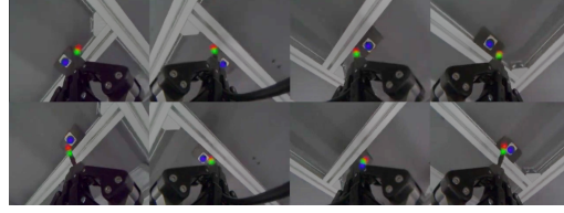
Figure 9: Model detections for two points in time. Each row is a single time-step.
