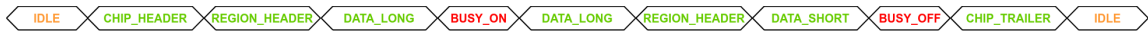
Figure 3: Example of a serial data stream from the Alpide chip. The busy words have priority, and can appear at an arbitrary point in the stream, even in the middle of a data frame (the green data words).
