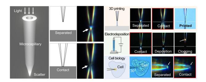
Principle and applications of KERI technology that uses light to determine microcapillary's contact in the nanoscale resolution. Credit: Korea Electrotechnology Research Institute
