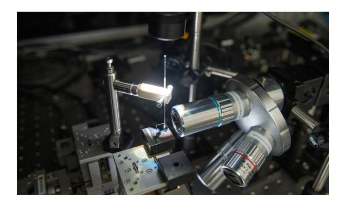
The visualization of microcapillary tips using a projection light to the back aperture for delicate contact of the tip surpassing the diffraction-limited resolution. Credit: Korea Electrotechnology Research Institu
