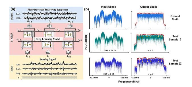
(a) Schematic diagram of the time-domain characteristics of fiber Rayleigh scattering restoration based on a deep learning model. (b) In the frequency domain, different network parameter settings result in differences in the restoration of fiber Rayleigh scattering. Credit: Science China Press
