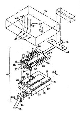
opening and chisels (46) cut areas over passages (37) on the base. Preset protuberances engage and set the arm when seating the frame so the dimple (31) engages and sets the switch (10) gap.
