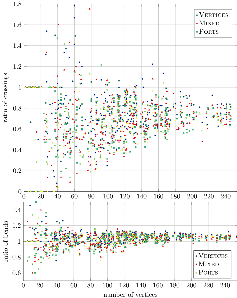
Figure 7.14: Comparison of the three crossing-reduction methods relative to KIELER. For handling local sources and sinks, we used RELPOS. In each color, each dot represents one of the 380 original cable plans.
