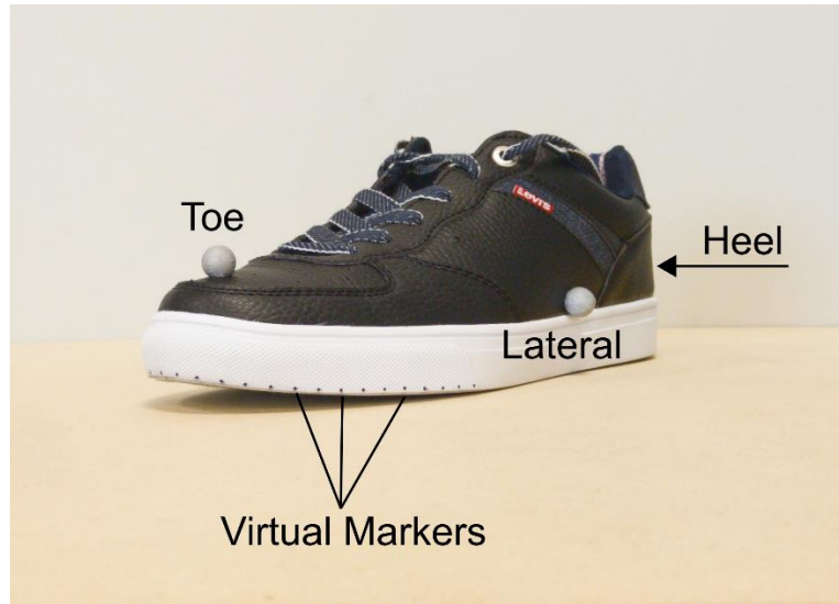
Figure 4. Photograph of the shoes worn by subjects showing the placement of physical markers and virtual markers. The positions of the virtual markers were defined within a shoe-fixed coordinate system defined using the three physical markers shown.
