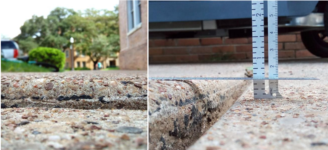
Figure 3 Left: Front-view of a representative tripping obstacle measured on the Texas A&M University campus; Right: Side-view of the same obstacle illustrating obstacle height measurement with a pair of rulers
