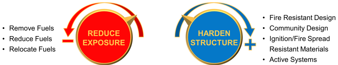
Figure 7. WUI fire hazard mitigation is a balance between two input dials—reducing exposure and increasing structure hardening.
