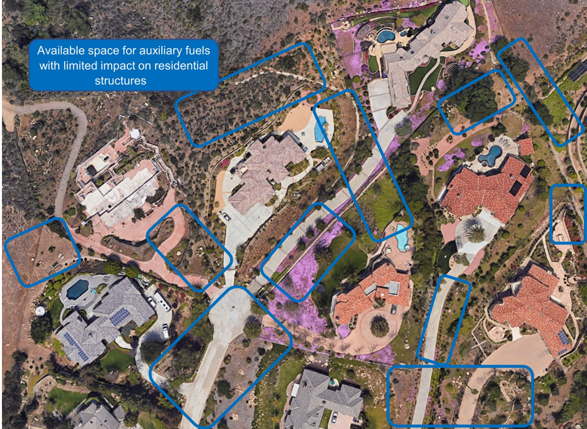
Figure 20. Scenario D, WUI Type 6. This community is characterized by large parcels with more extensive space available for auxiliary fuels. Avoidance of agglomeration of fuels within the outlined areas would influence the total number of auxiliary fuels allowed in these spaces.
