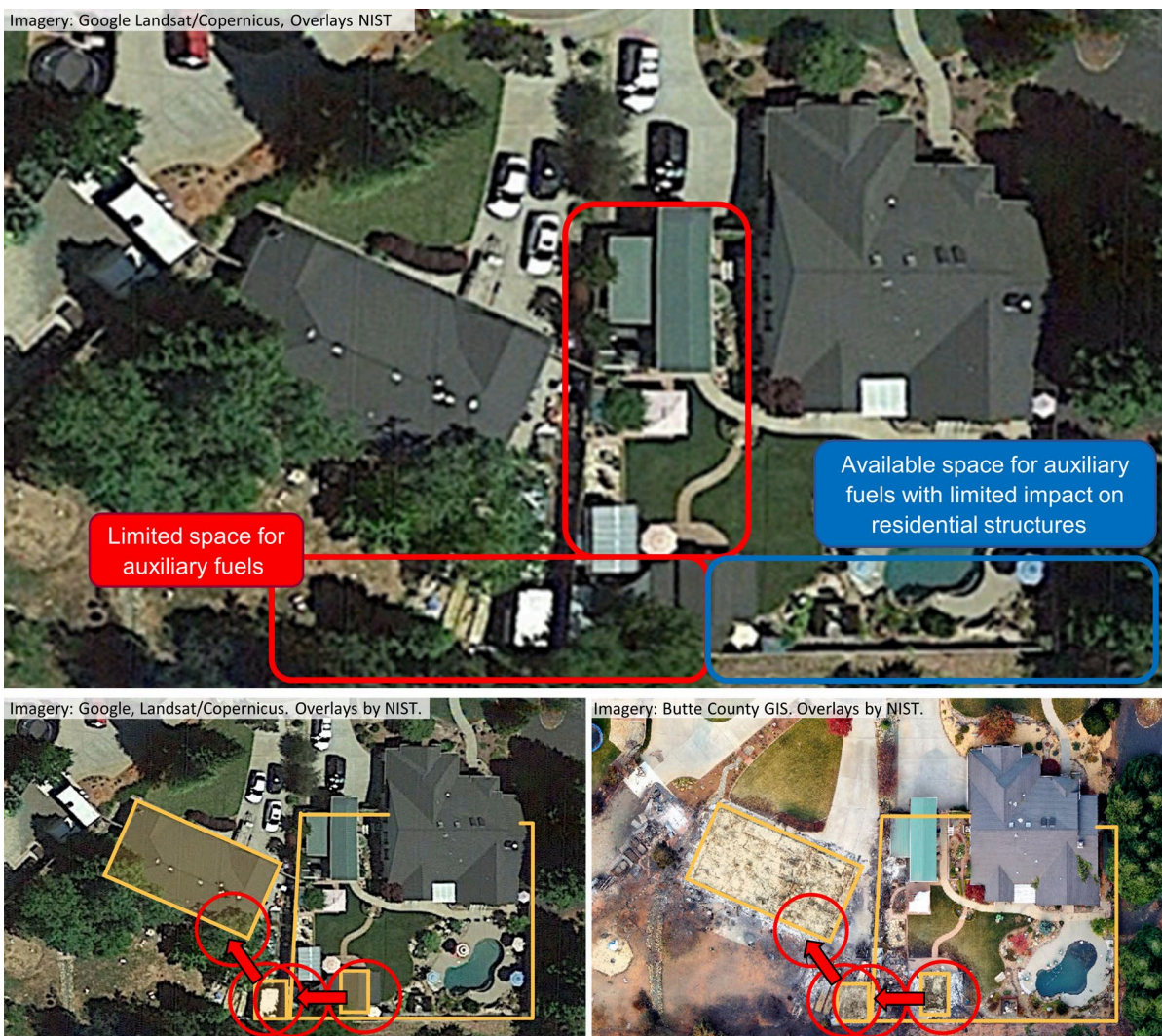
Figure 18. Scenario B, WUI Type 4. Moderate density interface. In some areas there is limited space for auxiliary fuels, shown by the agglomeration on the property boundaries (red highlights). The area highlighted in blue presents reduced impact on residential structures. The lower figures show before and after fire imagery with the actual fire spread pathway highlighted.
