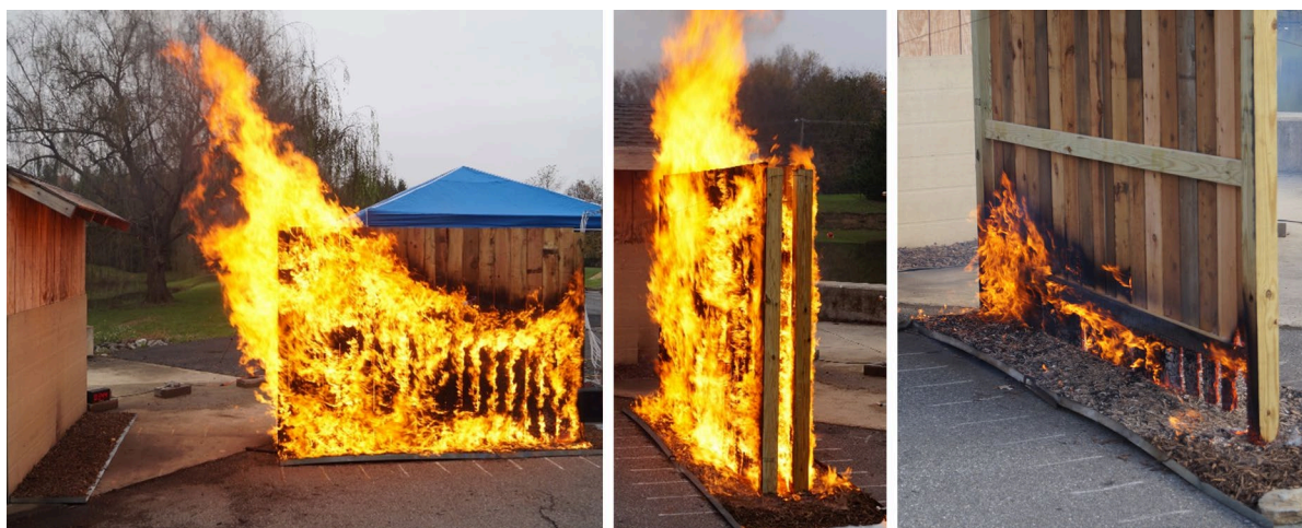
Figure 11. Parallel western red cedar fences burning with an applied wind of 13 mi/h (6 m/s) (left two images) compared to a single burning fence (right).
