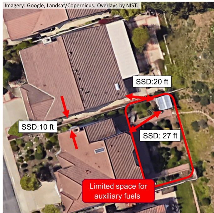
Figure 17. Scenario A, WUI Type 2. Small parcel with small SSD provides minimal space for auxiliary fuels. The shed is located closer to the neighboring residence than the owner's residence.
