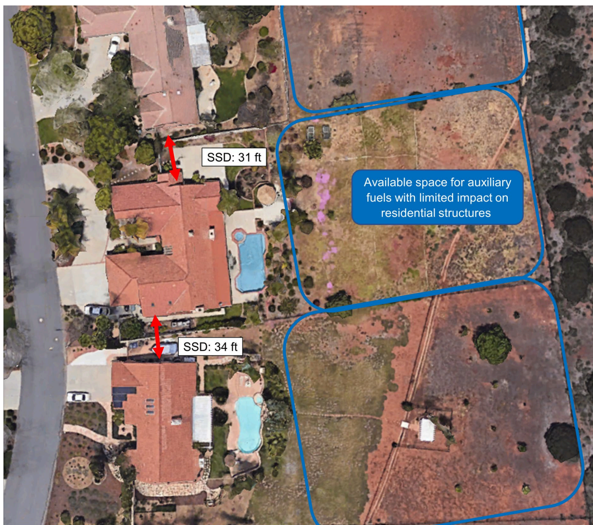
Figure 19. Scenario C, WUI Type 4 or Type 6. While the structures are placed on large parcels with extensive backyards, the primary structures are very large with considerably smaller SSD. Selective hardening may be required in this scenario despite the large parcels.
