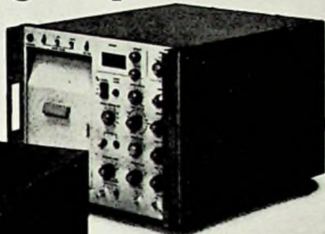
1806A Recording Oscillograph for Facsimile and X-Y-Y'-Z Plot Recording.
