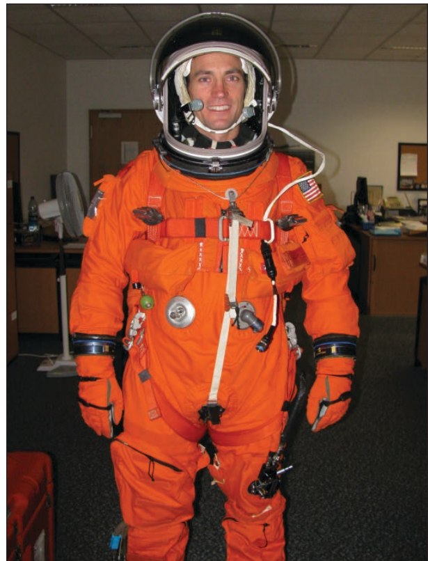
In 1994 the David Clark Company Model S1035 Advanced Crew Escape Suit began replacing the S1032 Launch Entry Suit.
