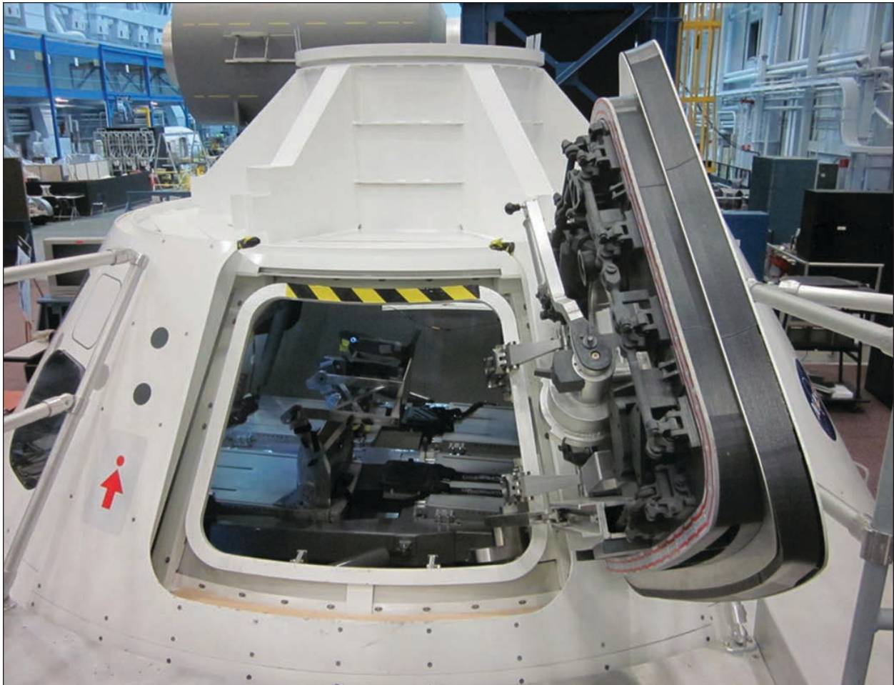
A mockup of the Orion Multi-purpose Crew Vehicle at the Johnson Space Center shows NASA's next-generation spacecraft, designed to carry humans beyond low Earth orbit to the moon, asteroids, and Mars.
