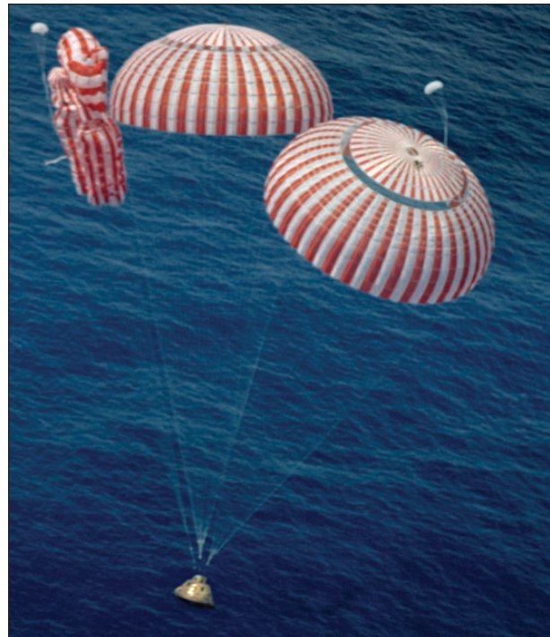
The Apollo 15 Command Module, with astronauts David R. Scott, commander; Alfred M. Worden, command module pilot; and James B. Irwin, lunar module pilot, aboard, nears a safe touchdown in the mid-Pacific Ocean to conclude a highly successful lunar landing mission. Although causing no harm to the crewmen, one of the three main parachutes failed to function properly. The splashdown occurred at 3:45:53 p.m. (CDT), August 7, 1971, some 330 miles north of Honolulu, Hawaii. The three astronauts were picked up by helicopter and flown to the prime recovery ship USS Okinawa, which was only 6 1/2 miles away.
