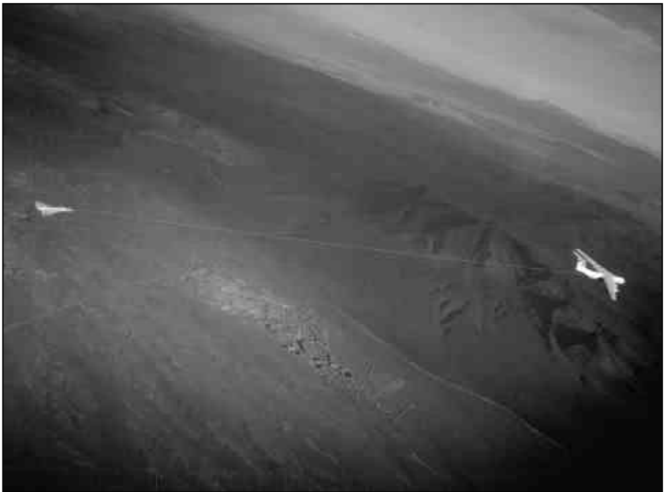
Side view of the C-141A towing the F-106. (NASA photo EC98 44415-19 by Jim Ross)
