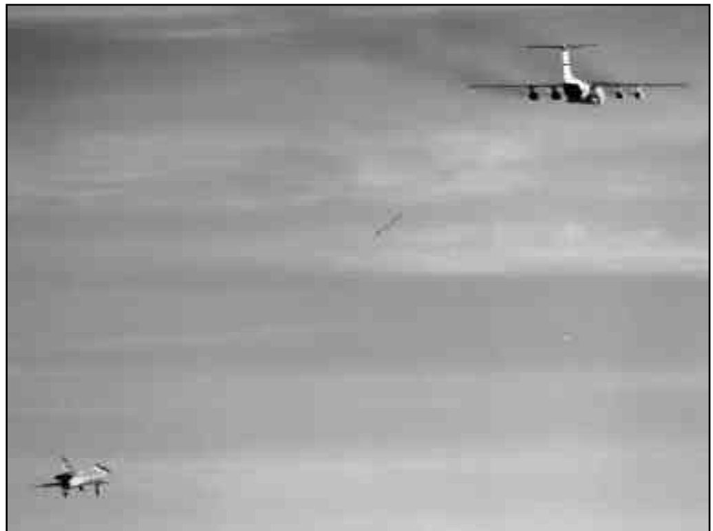
Eclipse project QF-106 and C-141A climb out under tow on first tethered flight, 20 December 1997. (NASA photo EC97 44357-13 by Tom Tschida)
