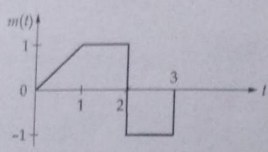
This signal is once used to frequency modulation of the carrier and once for phase modulation of the same carrier. Find the relation between  $K_p$  and  $K_f$  such that the maximum phase deviation in both the cases remains the same.
