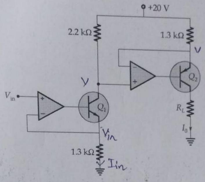
Vin=6V = Iin = 6V 1.3k2 = 4.615mA V = 20-4.615x 2.2 = 9.847V = 7.81mA For large 3:- Irz = 7.81mA Now for may R :-RL x 7.81x10 + 0.2 + 1.3x7.81 = 20
