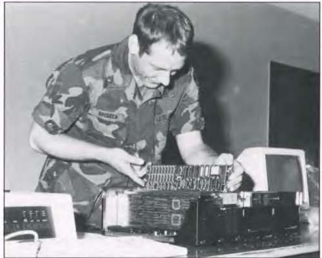
EASY DOES IT: Staff Sgt. Doug Brodeen reseats a circuit board after completing a diagnostic check of a Zenith Z248 computers.
